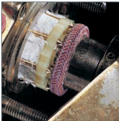
The Chesterton Stabilizer Cage can be used to maintain end ring loading in tough applications.
